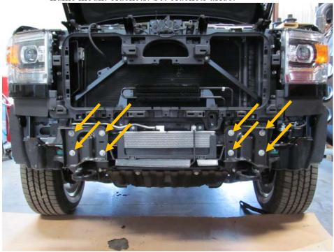
8. Using 18mm socket and wrench, remove OEM tow hook. Set tow hook aside. (both sides)
