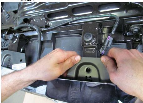
4. Using 15mm socket, remove 3 bolts from OEM bumper side brace in front of tire. Set aside. (both sides)
