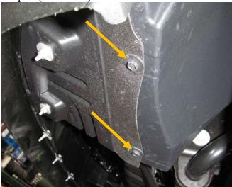
11. Using 15mm socket, remove three bolts from lower side bumper support. Set aside; it will not be reused. (both sides)
