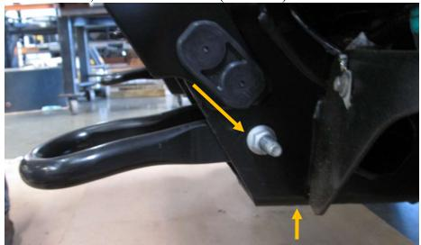
14. Using 18mm deep well socket, remove nuts on bolt strip. Remove strip and bumper mount. Set mount aside; it will not be reused. (both sides)
