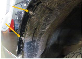
4. Using your hands, pull out on side of plastic fascia to disengage tabs from fender. (both sides)
