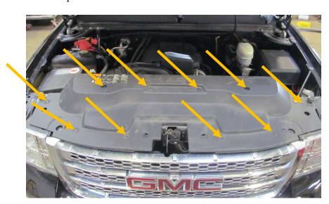
2. Using 10mm socket, remove four bolts attaching grill to truck.
