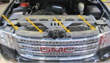
3. Using 7mm socket, remove two screws attaching plastic fascia to fender. (both sides)
