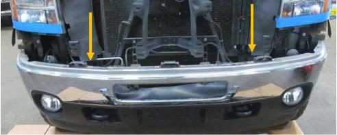
13. Use 18mm deep well socket and wrench to remove tow hook. Set aside; it will not be reused. (both sides)
