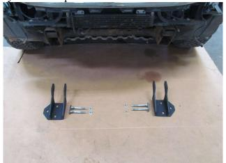
2. Install Hammerhead frame mounts on frame as shown using bolt strips. Do not fully tighten.
