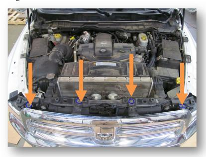
3. Using 18mm socket remove two nuts from the top of the bumper bracket. (both sides)
