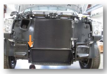
12. Remove bolt strip on Passenger side. (Bumper bracket will fall off once bolt strip is removed. Be mindful of any sharp edges on bracket)
