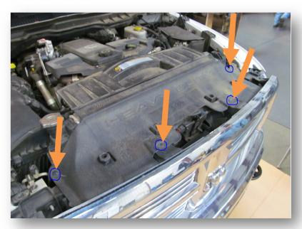
2. (Diesel only) Using a 10mm socket remove the grill by taking out four screws on top of grill. Pull gently on bottom of grill after screws are removed to release plastic tabs. Remove grill and set aside.
