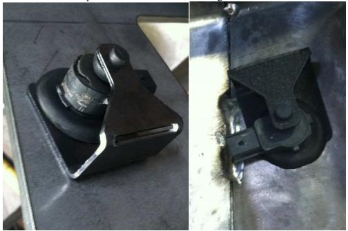
**6.** Install OEM sensor wiring harness and plug sensors in.
