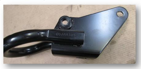
8. Using an 18mm socket remove two nuts. (both sides)
