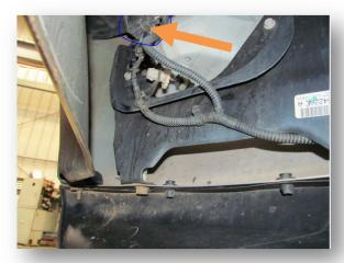
5. (Gas and Diesel) Using 18mm socket, remove two nuts that hold on the bolt strip (Be mindful of any sharp edges on bracket.) On diesel, carefully move one side of intercooler to ease in removal of bolt strip. (both sides) Carefully remove OEM bumper and set aside. Bolt strip will be reused to mount Hammerhead bumper.
