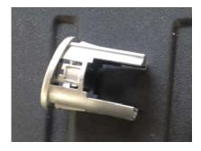
2. Install Hammerhead sensor solutions (601-56-2401) in two center holes of Hammerhead bumper. Then install OEM sensors and wiring harness. Make sure the sensors are oriented in the same way they were in the OEM bumper. NOTE: The plug will be horizontal.
