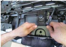
4. Using 15mm socket, remove 3 bolts from OEM bumper side brace. Set aside. (both sides)
