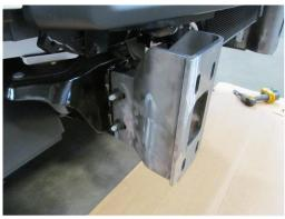
8. Attach Hammerhead bumper to frame mounts using eight ½" -13 bolts, sixteen ½" flat washers, eight ½" lock washers, and eight ½" nuts from Hardware kit 1.
