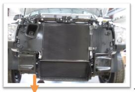
12. Remove bolt strip on Passenger side. (Bumper bracket will fall off once bolt strip is removed. Be mindful of any sharp edges on bracket)
