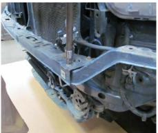
15. USING 10MM SOCKET REMOVE TWO NUTS AS SHOWN BELOW.
