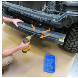
14. REMOVE SIX NUTS WITH 10MM SOCKET.
