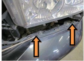
5. REMOVE 4 CLIPS IN THE CENTER OF OEM BUMPER.
