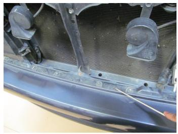
6. USING A 10MM SOCKET REMOVE TWO BOLTS UNDER THE HEADLIGHT COMPARTMENT (BOTH SIDES).
