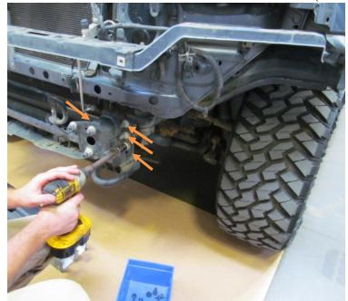
20. USING 17MM SOCKET REMOVE TWO BOLTS HOLDING ON OEM TOW HOOK.
