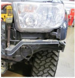
16. USING 10MM SOCKET REMOVE TWO BOLTS BELOW.
