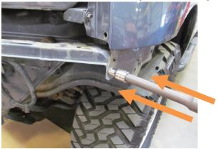
18. REMOVE ALL BUMPER SUPPORT STRUCTURE COVER FROM CENTER AND UNDERNEATH HEADLIGHTS.
