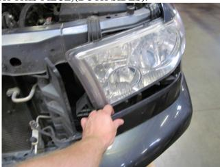
4. REMOVE TWO CLIPS FROM NEWLY EXPOSE COMPARTMENT (BOTH SIDES)
