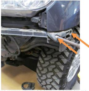
17. REMOVE TWO NUTS WITH 10MM SOCKET (BOTH SIDES)
