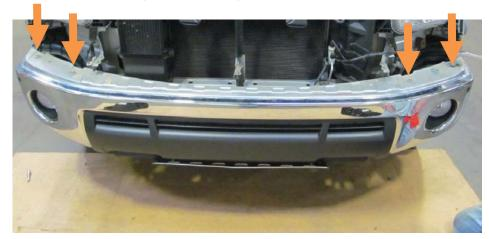
11. REMOVE ONE BOLT USING 12MM SOCKET UNDERNEATH OF CHROME BUMPER.
