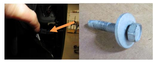
8. Carefully pull plastic OEM bumper downward and toward the front of truck to dislodge plastic upper fascia from vehicle. Remove and set aside.
