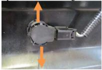
4. Now you can carefully remove the wiring harness and sensors from OEM bumper.
