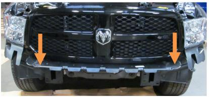
11. Using 10mm socket remove three bolts holding side bumper support. Remove side bumper support and set aside. (both sides)
