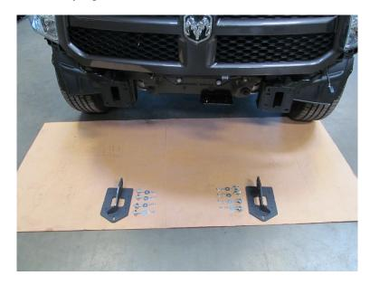
7. In this step you will use hardware kit #64. Using six ½"-13 x 2.00" bolts, six ½" flat washers, six ½" lock washers, and weld nut tabs (601-56-2868) fasten Hammerhead bumper to Hammerhead frame mounts. Align bumper to center of vehicle, and tighten all hardware using ¾" socket.
