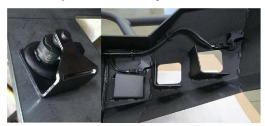
5. Install OEM sensor wiring harness and plug sensors in.
