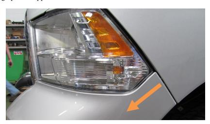
9. Using 10mm socket remove two bolts holding on center bumper support structure. (both sides)
