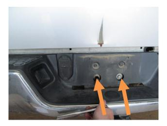
5. Using 15mm socket, remove two bolts holding on OEM bumper. (both sides)
