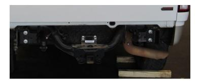
8. Install provided 1/8" thick washer in bumper's center mount and secure with OEM bolts or nuts. (Slide washers in from the side.) Do not fully tighten.
