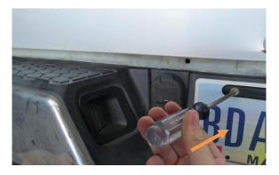
4. Behind the license plate there are either two bolts or two nuts depending on year model. Use 15mm socket to remove both of them.
