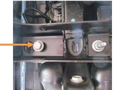
6. Loosen two receiver mount bolts. Hint: Use a 21mm wrench to hold the nut and use a 10mm socket to turn the bolt.
