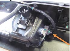
10. Remove OEM spare tire access housing. Pry back metal fingers on ring and remove plastic insert.
