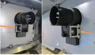
3. Install OEM spare tire access housing.
