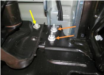
5. Remove bolt in receiver hitch with 21mm socket. (both sides)
