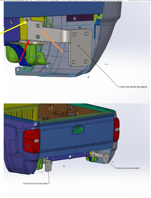
7. Use hardware kit #1 for this step. Install bumper on Hammerhead frame mounts with eight ½"-13 x 2" bolts, 16 flat washers, eight lock washers, and eight nuts. These mounts will set the left to right and the up and down adjustment of the bumper. Make sure to check tailgate clearance before tightening bolts.
