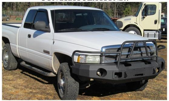
(Hammerhead X-Series Winch Bumper shown. Your bumper's final appearance will differ slightly)
