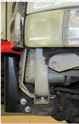
FIGURE 8: OUTSIDE VIEW OF FRAME MOUNTS
