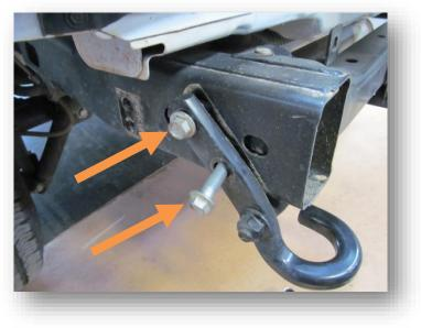
Figure 7 Using 19 mm socket remove single bolt holding on tow hook on the bottom of driver side frame rail. See figure 8. 8.
