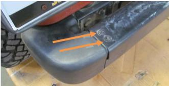
3. Using an 18mm socket, remove bottom bolt attaching bumper to frame. (both sides)
