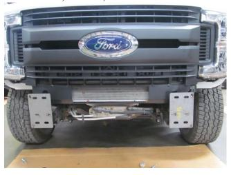
4. Layout weldnut tab 5 and hardware from kit # 97 as shown.
