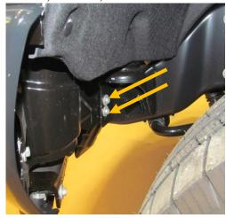
3. Using 18mm socket, remove eight bolts attaching the bumper to the frame. Remove bumper and set aside. It will not be reused.
