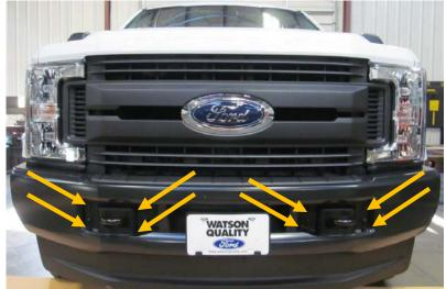
4. Using 18mm socket, remove four bolts attaching tow hook to frame. Set aside; it will not be reused. (both sides)
