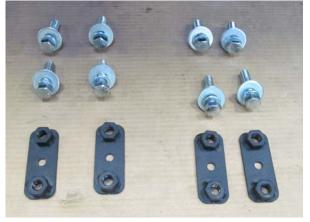
5. Using a hoist or a few friends, attach bumper to frame mounts using hardware kit #97. Insert bolts from frame mount side and use weldnut tabs on inside of bumper. Start all bolts before aligning bumper. Align bumper a minimum of 3/8" below headlights. When truck flexes offroad, this distance allows your bumper and body to have clearance. Tighten all bolts on bumper and frame mount with 3/4" socket and wrench.
