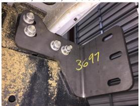
9. Using hardware kit # 53 and two weldnut tabs, attach bumper to HH frame mounts. Do not fully tighten.
