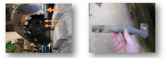
3. Using a 21mm socket remove two nuts from the bolt strip attaching the bumper to the frame of vehicle. (both sides)
