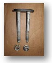
4. Using 18mm socket and wrench remove the bolts attaching the tow hook to the frame. Remove tow hook and set aside. (both sides).
