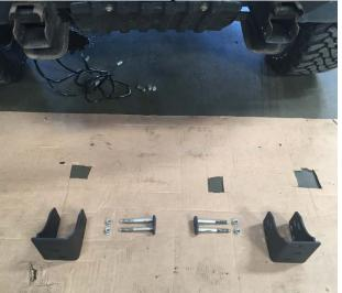
3. Install frame mounts with OE bolt strips and OE tow hook bolt. Do not fully tighten.
