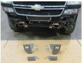
2. Install Hammerhead frame mounts (0934 & 0935) on top OE bumper mounts using OE hardware. Do not fully tighten.
