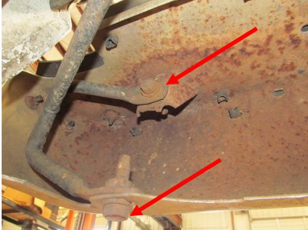
2. Using an 18mm socket, remove the 4 bolts that hold the bumper to the frame. (2 on each side)
