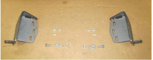
3. Attach HH frame mounts to truck frame with OE hardware. Do not fully tighten.
