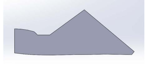
6. Align template to line where plastic OE bumper and metal fender meet. Use some tape to keep it in place while you trace the bottom of the template with a permanent marker. After tracing the final cut line, measure down 3/16" and make another line for your initial cut line.
