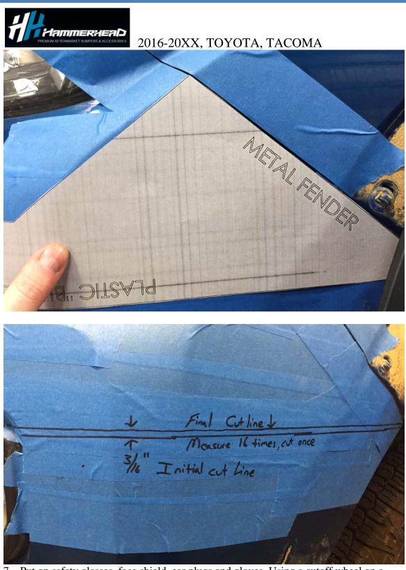
7. Put on safety glasses, face shield, ear plugs and gloves. Using a cutoff wheel on a electric grinder or air die grinder, cut initial line. This will separate the bottom of the bumper side from the top. Do not allow the cutoff wheel to go more than 1/8" deeper than the plastic bumper. This could damage the metal fender or plastic retainer clip near the tire. The bottom of plastic retainer clip will be cut off after the OE bumper is removed.
