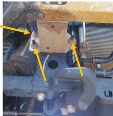
20. Using 17mm socket, remove two bolts attaching OE tow hook to frame. Remove hook. Remove one bolt attaching fender extension to frame. (both sides) Remove fender extensions.
