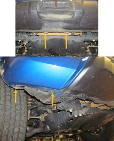
12. Unplug OE fog lights. Plug is located in center of truck where the bottom of the grill
