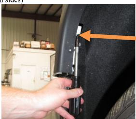
4. Pull out on edge of plastic trim to release the tabs as shown. Pull in direction of arrows. (both sides) (2014-2015 shown)
