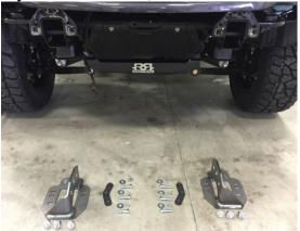
3. Install Hammerhead frame mounts with OEM hardware and loosely tighten. Use the top holes in the mounts.
