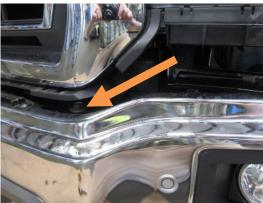
10. Remove six bolts holding on OEM frame flanges to frame with 15mm socket.
