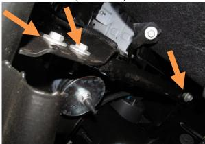
9. Remove OEM bumper bolt with 18mm wrench. (both sides) Remove OEM bumper and set aside.
