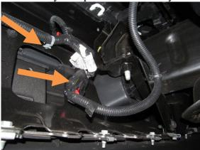
7. Remove OEM bumper bolt behind bumper with 18mm socket. (both sides)
