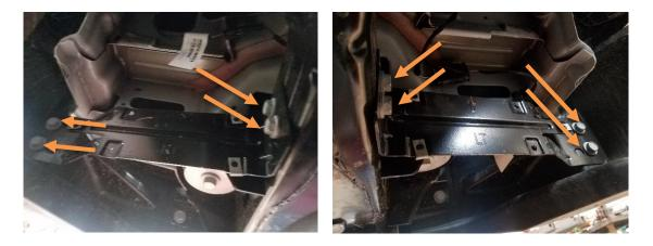
3. Remove the 2 bolts on each side that attach the bumper. Use a 15mm socket.
