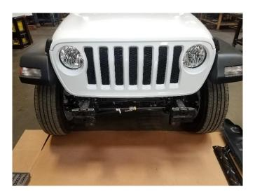
7. Remove the plastic cover on each side of the front bumper using the torx 20. There are 7 screws.
