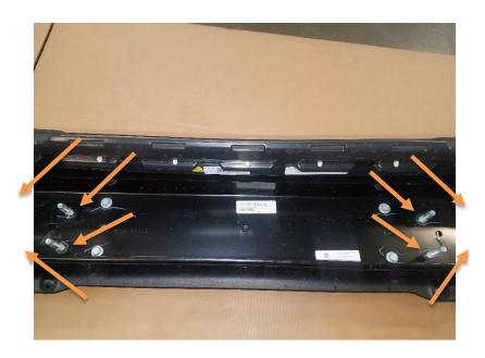
11.Remove the 4 bolts holding on the metal plate with a 15mm socket. Remove the metal plate and set aside.
