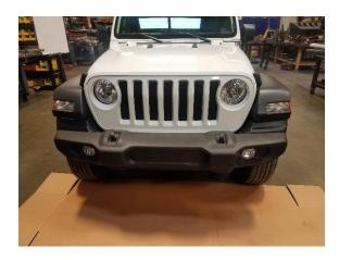
1. Remove 8 plastic clips from front of OE "skid plate". Using the 8mm socket, remove the two bolts from the bottom then remove the skid plate.
