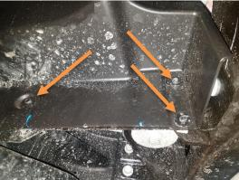
2. Remove the 4 bolts attaching the side reinforcement with a 15mm socket. Remove the plate from both sides.
