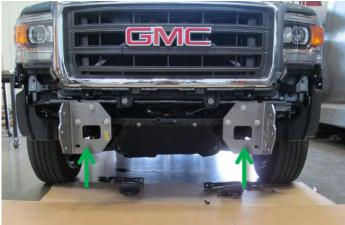
3. Install Hammerhead lower frame mounts. Do not fully tighten. Use OE hardware for through frame bolt.
