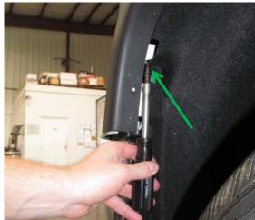
4. Once all screws have been removed from both sides, pull out on the edge of the plastic trim to release the tabs. Pull in the direction of the arrows in the pictures below.
