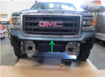
5. Using a hoist or a few friends, attach bumper to frame mounts using hardware kit #1. Start all bolts before aligning bumper. Leave a minimum of 3/8" space between bumper and truck body. When the truck flexes off-road, this distance allows your bumper and truck body to have clearance. Tighten bolts with 3/4" socket and wrench. Tighten frame mount bolts at this time. Use suggested torque values from page one.
