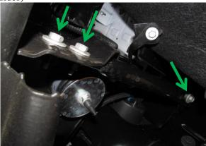
9. Remove OE bumper bolt with 18mm wrench (both sides)
