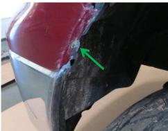
2. Using an 8mm socket, remove the bolt attaching the inner fender to the fender. This bolt will be re-used. (both sides)
