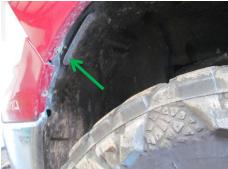
3. Using 10mm socket, remove bolt attaching plastic fascia to fender. Push inner fender towards the frame and down to gain access to the bolt.
