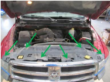
9. Using a 10mm socket, remove four screws attaching the grill to the frame. They are located on top of the grill.
