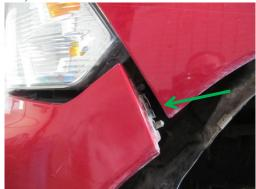
5. Unplug fog lights (if applicable). The plug is located above the fog light in front of the left side tire.
