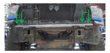
13. Using 10mm socket, remove one bolt attaching side plastic fascia support to frame. Remove support and set aside. (both sides)
