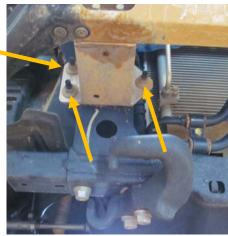
20. Using 17mm socket, remove two bolts attaching OE tow hook to frame. Remove hook. Remove one bolt attaching fender extension to frame. (both sides) Remove fender extensions.
