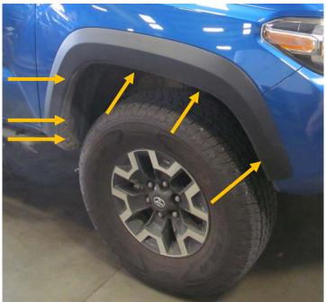
2. Starting at the front of the truck, gently pull out on the fender flare to disengage the plastic clips. You will need easy access to the OE bumper under the flare. You can remove the entire flare if you want.
