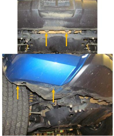
12. Unplug OE fog lights. Plug is located in center of truck where the bottom of the grill was.
