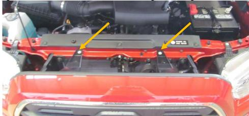
9. Using trim tool, remove two plastic clips attaching grill to headlights. NOTE: Pry up on center of clip.
