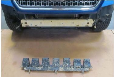
19. Using 14mm socket, remove six bolts attaching OE crash bar to frame. (three per side) Remove OE crash bar. NOTE: If you can't get the bar off, loosen three bolts on one side of the crash bar extrusion.
