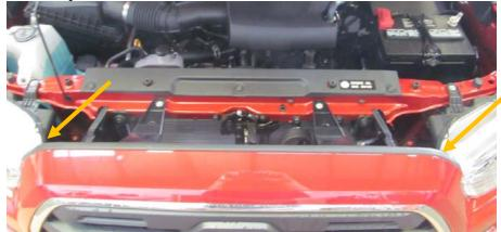
10. Gently pull out on grill near headlight to release plastic tabs. (both sides) Set grill aside; It will be reused.
