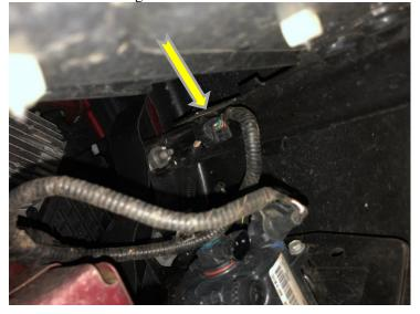
3. Using a 12mm socket, remove the mount bolts attaching the bumper side supports to the frame. These supports are located in front of the front tires. (Both sides)
