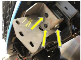
5. Using a hoist or a few friends, attach bumper to frame mounts using hardware kit #58. Start all bolts before aligning bumper. Leave a minimum of 3/8" space between bumper and truck body. When the truck flexes off-road, this distance allows your bumper and truck body to have clearance. Tighten bolts with 3/4" wrench or socket. Tighten frame mounts at this time. Torque to specs on page one.
