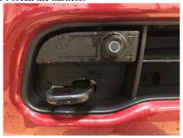
5. Using a 14mm socket, remove the 3 OE bumper mounting bolts. Set these bolts aside, they will be used again. (Both Sides)
