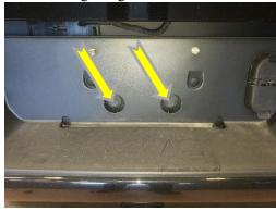
5. Remove the two nuts holding the bumper to the frame on both sides. You will use a 16mm socket.
