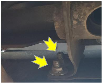
4. Align and level bumper with the truck. Tighten the center bolts with a 15mm socket and bumper mount bolts with a 34 wrench and socket. Install license plate mounting kit and license plate on bumper.
