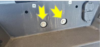
3. Install (4) bolts, (8) flat washers, (4) lock washers, and (4) hex nuts from hardware kit #4 into the bumper mounts.
