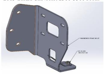
8. Install Hammerhead bumper on frame mounts using bolts, flat washers, lock washers, and nuts from Hardware Kit#1 and 3/4" wrench and socket.
