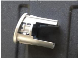
2. Install Hammerhead sensor grommets in two center holes of Hammerhead bumper. Then install OEM sensors and wiring harness. Make sure the sensors are oriented in the same way they were in the OEM bumper.
