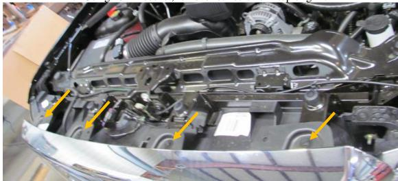
3. Gently pull out on grill to remove. Start at top by pulling up and then out. Then pull out on bottom. Gently set aside. It will be reused.
