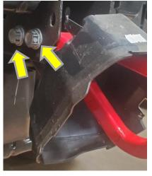
13. Using a 15mm socket, remove (6) bolts from the bumper mounts. Set hardware aside to be reused. Remove bumper mounts from truck.
