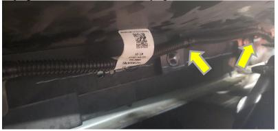
10. Using a 10mm and 15mm, remove (6) bolts from the outer bumper supports and (4) bolts from inner bumper supports.
