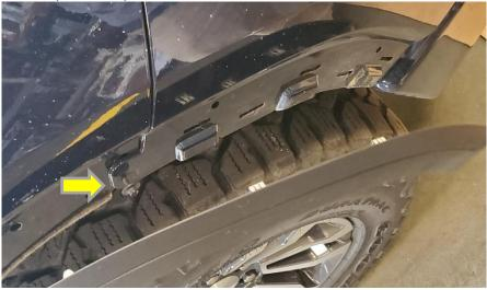
4. Using a T-15 torx, remove the bolts holding the inner fender to the front bumper and valence.
