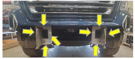
4. Layout hardware from hardware kit #1. Use (6) bolts, (6) flat washers, and (6) flat washers with (2) weld nut tab 3's.
