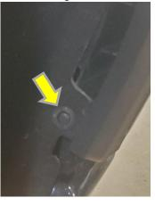
5. Using a 10mm removed the (4) bolts holding the top of the grill in. Pull up on tabs to release
