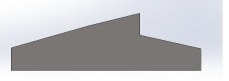
8. Align the paper cut template on the vehicle as shown below. Do this on both sides. The bottom of the cut template will help draw a straight line across the corners of the bumper.
