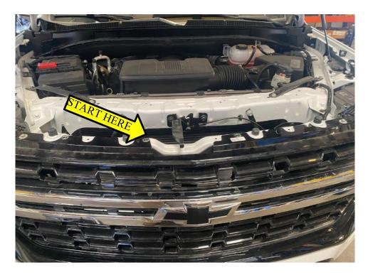
18. Using a 7mm wrench or socket reinstall the (6) flange bolts (3 per side) from the fender wheel well to the bumper. Followed by installing the (6) T15 (3 per side) screws in the inner fenders as well. NOTE: there will be some hardware not reused\*\*
