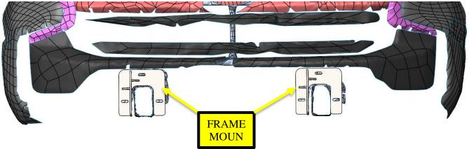
3. Next, install the bumper using Hardware kit #58 and both Weldnut tab #3. Hand tighten hardware so the bumper can easily be adjusted and moved. Pull bumper so that it is as far forward in the frame mount slots as possible. Push bumper downward so that it is in the lowest adjustment position. Note: Make sure bumper is level at this point.
