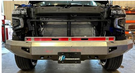
4. Using a tape measure, take measurements from the ground to the top of the bumper. Measure each spot marked below and record the measurements. The measurements should be consistent across the top of the bumper from left to right.
