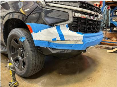
9. Using the cut template and the measurements taken in step. 4. Draw a line across the front of the vehicle for the 1<sup>st</sup> cut. Take your time during this step. Measure many times and double check the cut line before proceeding to step 9.
