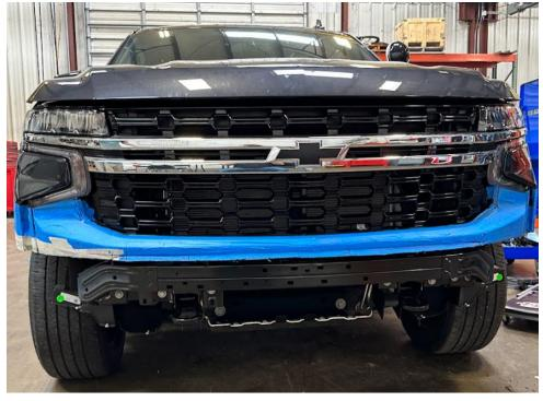
11. With the 1<sup>st</sup> cut complete. Remove the center trim left over.
