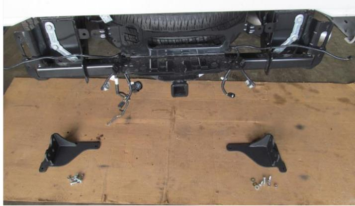
8. Using six ½"-13 carriage head bolts, six ½" flat washers, six ½" lock washers, and six ½"-13 nuts fasten Hammerhead bumper to Hammerhead frame mounts. Align bumper horizontally and vertically and tighten nuts using ¾" socket. Note: Open tailgate slowly to ensure minimum of 3/8" clearance below tailgate and minimum of 3/8" clearance from truck body. NOTE: If bumper is too low when pushed all the way up, receiver hitch hardware can be loosened and hitch/bumper can be moved up.
