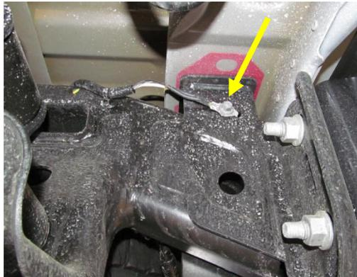
4. Using a 21mm socket, remove six bolts attaching OEM bumper/receiver hitch to frame. Remove and set aside face down on foam or cardboard.
