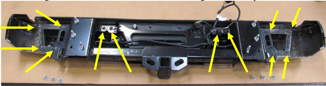
10. Using a 13mm wrench, remove two bolts attaching metal portions of bumper to receiver hitch. They are located behind the OEM license plate lights. Note: They are difficult to remove. Remove the spring nuts after removing the bolts. They will rattle if not removed.
