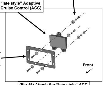
(Fig 15) Attach the "late style" ACC sensor to back of Adapter Plate
