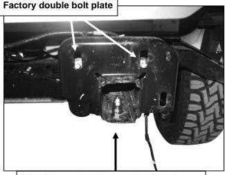
(Fig 5) Insert double nut plate into frame
