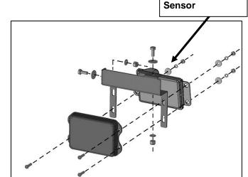
(Fig 17) Attach early style ACC sensor to the back of the ACC Mounting Bracket
