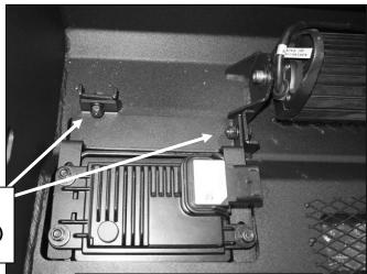
(Fig 19) ACC assembly attached to the back of the Bumper
