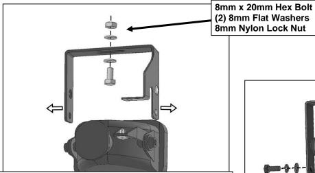
(Fig 12) Optional OEM fog light installation (light not included). Attach driver/left Upper Bracket to the slot in top of the opening. Carefully spread sides to slide OEM fog light into position in pivot holes
