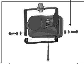
(Fig 13) Attach lower U Bracket to Upper Bracket. Reuse factory adjustment hardware (screw, spring and plastic nut)
