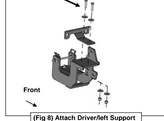
(Fig 8) Attach Driver/left Support Bracket to top of Frame Bracket
