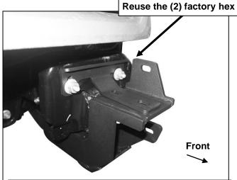
(Fig 9) Attach the Driver/left Support Bracket to the frame using the (2) factory flange nuts
