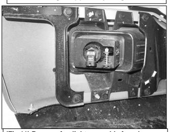
(Fig 11) Remove fog light assembly from bumper
