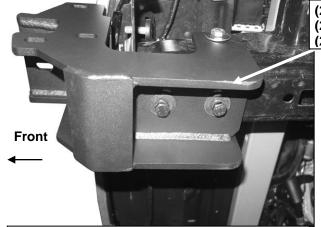
(Fig 7) Driver/left side Frame Bracket installed
