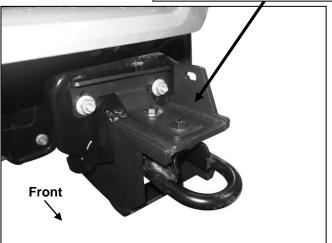
(Fig 10) Driver/left side Support Bracket attached to Frame Bracket with tow hook
