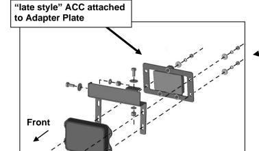
(Fig 16) Attach late style ACC assembly to the back of the ACC Mounting Bracket
