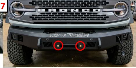
Adjust Fitment of Bumper and Tighten All Nuts and Bolts.
