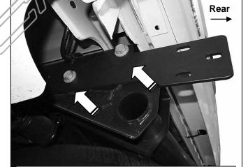
(Fig 2) Reuse factory bumper bolts to attach Frame Bracket to side of frame, (driver side)
