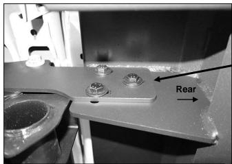
(Fig 4) Attach Bumper to inside of Frame Brackets (driver/left side pictured from below)
