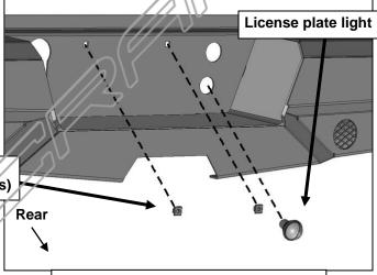
(Fig 5) Attach License Plate Light and (2) Plastic Plugs for the license plate
