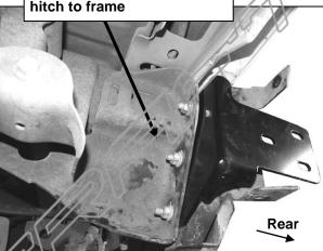
(Fig 8) Driver/left side Mounting Bracket with receiver hitch attached to frame
