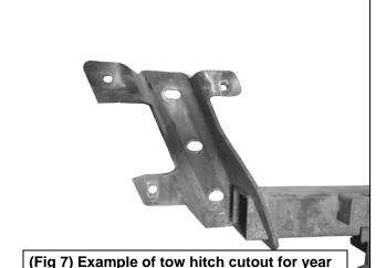
(Fig 7) Example of tow hitch cutout for year models 06-08 re-using factory receiver hitch
