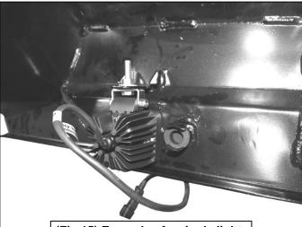
(Fig 15) Example of a single light attached to the mounting tab.
