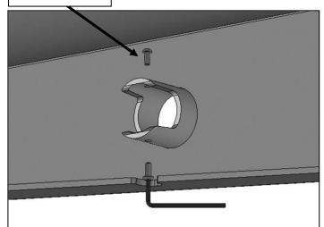
(Fig 12) Push sensor into mounting sleeve. Use 4mm Screws to lock sensor in place.
