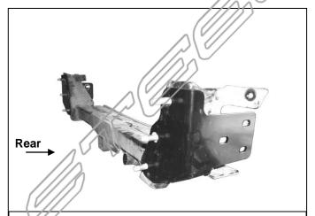
(Fig 5) On models with factory receiver hitch, slide Mounting Bracket up against the hitch. Insert triple bolt plates through hitch and Brackets.
