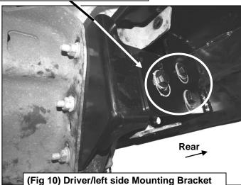
(Fig 10) Driver/left side Mounting Bracke with receiver hitch attached to bumper
