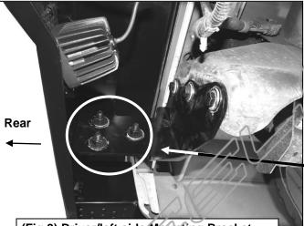
(Fig 9) Driver/left side Mounting Bracket without receiver hitch attached to bumper
