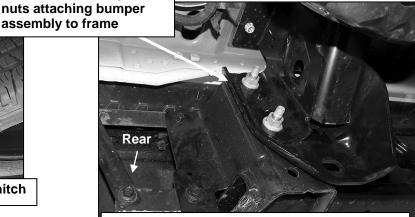
(Fig 3B) Remove the factory hex nuts attaching bumper assembly to frame. STD tow package model pictured (no receiver hitch)
