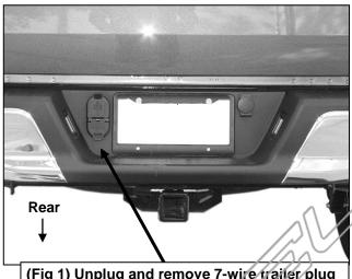
(Fig 1) Unplug and remove 7-wire trailer plug
