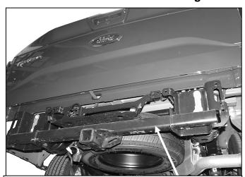
(Fig 13) Reinstall integrated receiver hitch/bracket assembly on models with "HD Towing" package
