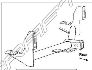
(Fig 5) Example of "Max Duty" OE style receiver hitch
