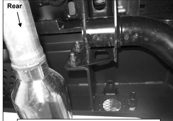
(Fig 13) Driver/left side of the Rear Bumper attached to the factory hitch
