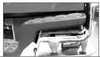
(Fig 6A) Remove center plastic piece on top of the bumper
