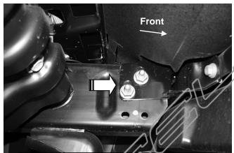
(Fig 3) From behind bumper, remove the hex nuts, (arrow), attaching the bumper bracket to the double colt plate (driver/left side pictured from behind bumper)
