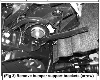
**WARNING!** Do not crawl under bumper or remove bumper bolts unless the bumper is properly supported on blocks or stands or the bumper may fall.
