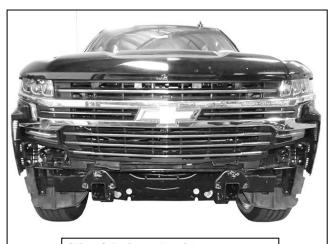
(Fig 8) Reinstall grille and cover
