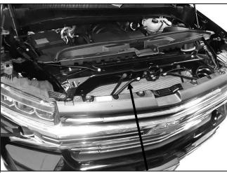
(Fig 1) Remove cover and screws attaching grille
