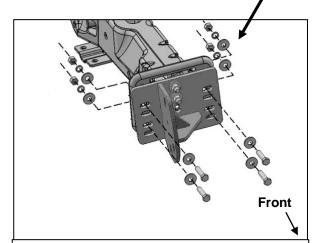
(Fig 15) Attach Frame Bracket frame. 2005-07 Driver/left side illustrated for example
