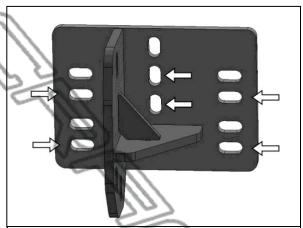
(Fig 12) On 1999-04 models, use the lower mounting slots in the driver/left Frame Bracket as illustrated, (arrows)
