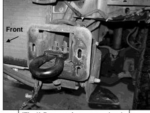
(Fig 6) Remove factory tow hook
