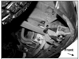
(Fig 2A) On 1999-04 Models equipped with lower cross member bumper support, remove crossmember.
