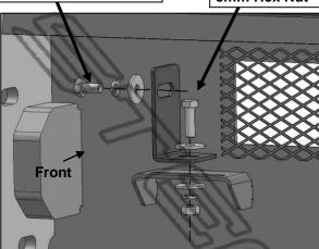
(Fig 18) Attach Left/Right LED Brackets to tabs on back of Bumper (left side illustrated)
