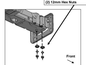
(Fig 10) Insert the Driver/left Support Bracket into the frame. Insert (2) Single Bolt Plates into and down through the holes in the frame.
