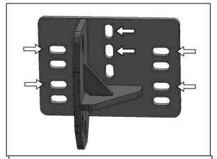
(Fig 13) On <u>2005-07</u> models, use the upper mounting slots in the driver/left Frame Bracket as illustrated, (arrows)
