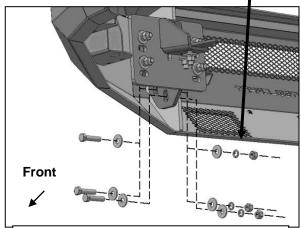
(Fig 19) Attach Driver/left side of Bumper to inside of Frame Bracket
