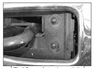
(Fig 4) Remove factory bumper bolts
