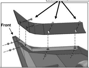
(Fig 16) 2005-07 models only, attach Fill Panels to top of Bumper. Driver/left illustrated
