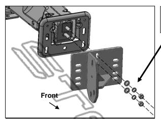
(Fig 14) Attach Frame Bracket to Bolt Plate in Support Bracket. 2005-07 Driver/left side illustrated for example
