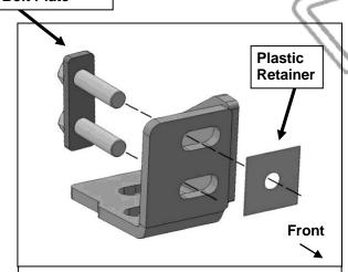
(Fig 7) Driver/left Support Bracket with (1) Insert Double Bolt Plate through back of driver/left Support Bracket. Thread Plastic Retainer onto Bolt Plate to hold in place
