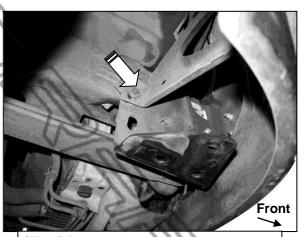
(Fig 3) Remove outer bumper supports attaching ends of bumper to frame (passenger/right side pictured)
