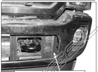
(Fig 3) Remove factory bumper bolts
