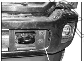
(Fig 3) Remove factory bumper bolts
