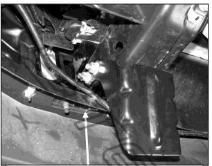
(Fig 1) Unplug driver/left side fog light wire harness (pictured from behind bumper)
