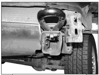
(Fig 5) Remove driver/left tow hook
