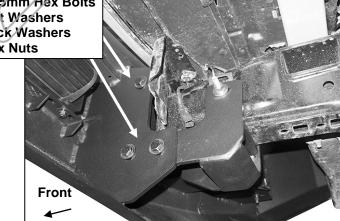
(Fig 14) Attach Bumper to Frame Brackets. Passenger/right side pictured from below
