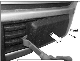
(Fig 1) Carefully pull plastic bumper pad off of bumper
