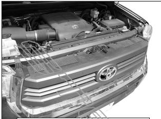
(Fig 1) Remove plastic cover and grille
