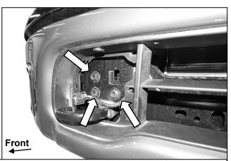
(Fig 2) Plastic cover removed. Remove the factory bolts from the mounting bracket to remove the bumper (Passenger/Right side shown)
