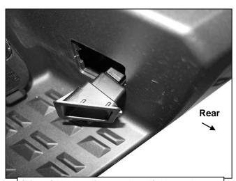
(Fig 16) Unplug license plate lights and trailer connector. Remove lights and
