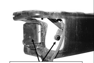
(Fig 10) Remove sensors and wiring harness. Rear Cross Traffic Alert (RCTA) and parking sensors pictured
