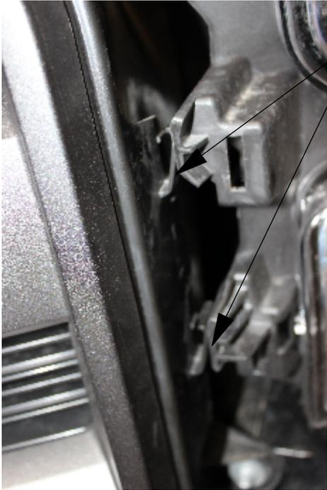
**Step 4** Grille retaining tabs two per side
