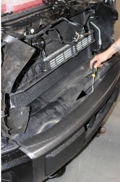
**Step 5** remove plastic cover attached to back of bumper
